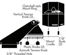
**WARNING:** Rotating the Tele-Pod head while the azimuth tension knob is tightened could cause the azimuth bearing to unscrew and separate.
